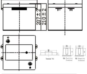
Lenght $281\pm 2mm(11.06inches)$ Width $267\pm 2mm(10.51inches)$ Container Height $207\pm 2mm(8.27inches)$ Total Height $210\pm 2mm(8.15inches)$
